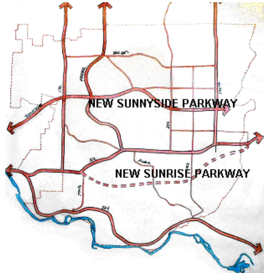
First concept for new street system. Thick red lines denote major streets; thin red lines denote medium capacity streets; dotted line denotes a possible Southern Parkway alignment. The agricultural grid and the 600 X 600 ft. block increment was used as a basis for expanding the street network. Existing east-west connections along the existing 212 and 224 corridors are supported by an additional east-west connection to the north of highway 212. North-south routes are strengthened to accommodate the increase in demand and to increase interconnectivity through the site.
